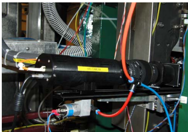
Fig. 2 The fast camera for discharge overview, developed especially for the COMPASS tokamak, mounted with optics on the toroidally oriented port
