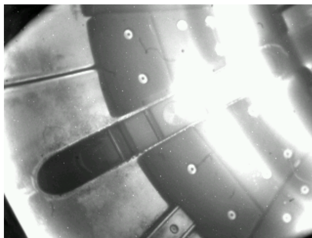
Fig. 5 Observation of the divertor leg traces using the slow CCD camera on the COMPASS tokamak in the shot #3329. Exposure time is 100 ms, starting at 1162 ms
