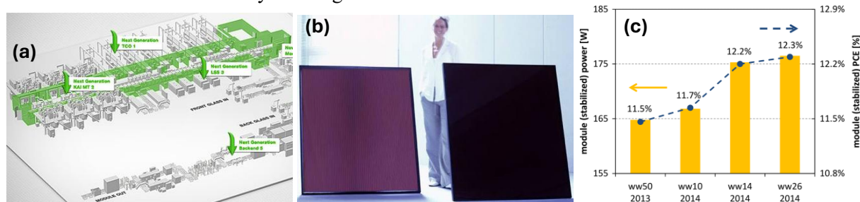
Fig.1. Layout of module production fab (a), a-Si and tandem solar panels (b), Efficiency improvements (c).
