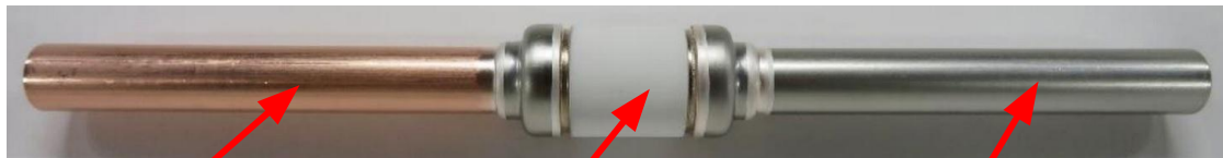
copper side el. ceramic breaks Stainless steel part
